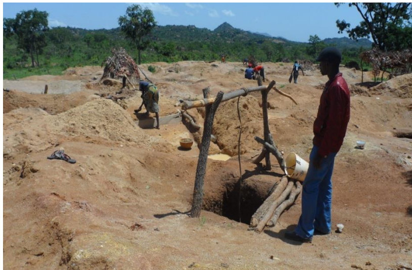
Plate 2: Local underground mining (loto mining) of topaz and cassiterite within the Jarawa-biotite-granite alluvium at Zebir-Nabar.
