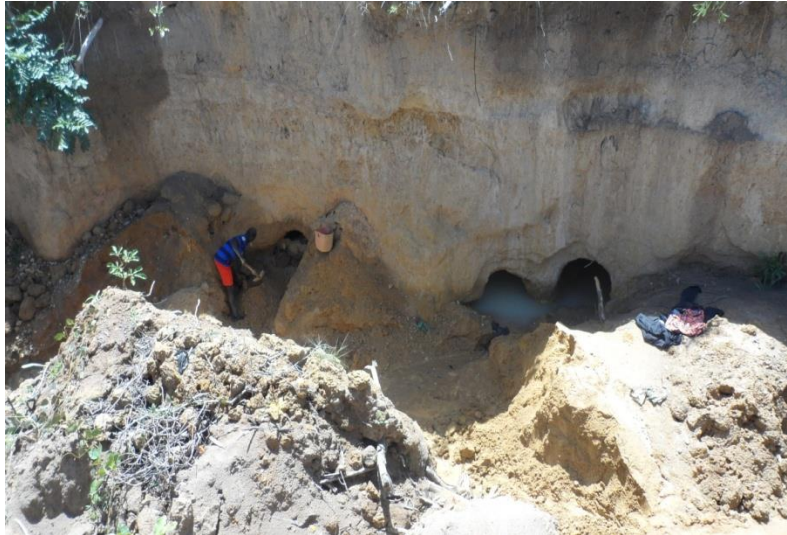
Plate 1: A picture showing the local underground mining (loto mining) of topaz in Zabir-Nabar, a part of the study area within the Jarawa-biotite-granite.
