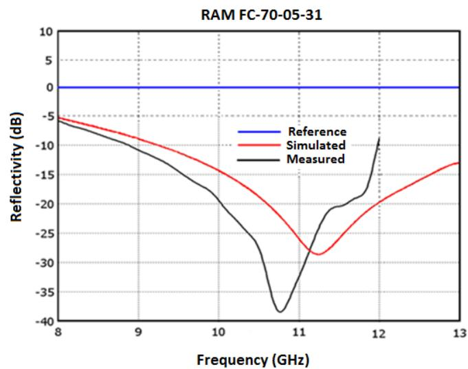
Fig. 6. The reflectivity curve of the RAM FC 70-05-31 used in the study of RCS reduction.
