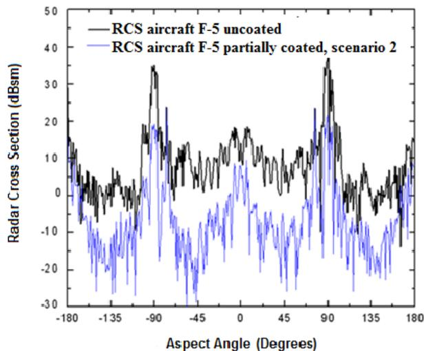
Fig. 9. Comparison between the RCS of the F-5 modified at 11 GHz, partially coated and uncoated with RAM. (scenario 2).
