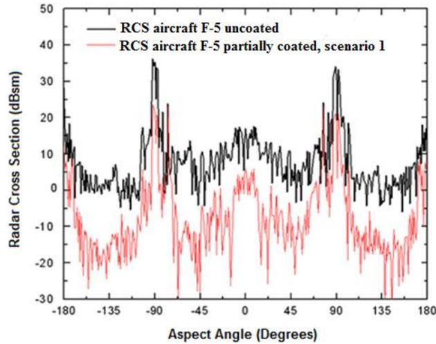
Fig. 7. Comparison between the RCS of the F-5 modified at 10 GHz, partially coated and uncoated with RAM (scenario 1).
