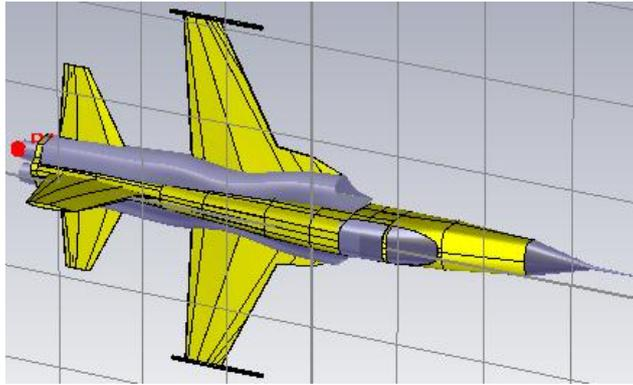
Fig. 4. Aircraft F-5 partially coated with RAM, scenario 3.
