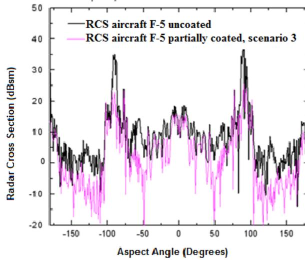
Fig. 10. Comparison between the RCS of the F-5 modified at 11 GHz, partially coated and uncoated with RAM. (scenario 3).
