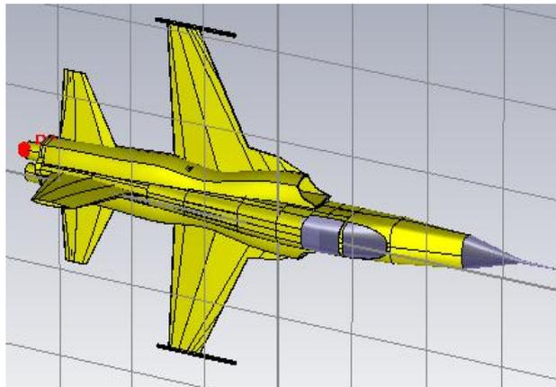
**Fig. 2. Aircraft F-5 partially coated with RAM, according to scenario 1.**
