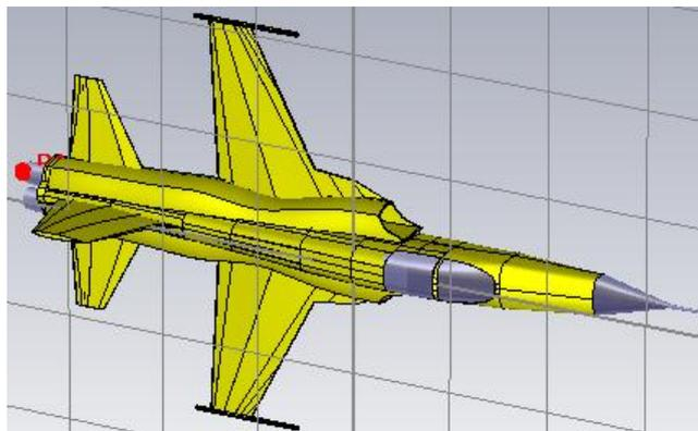
**Fig. 3. Aircraft F-5 partially coated with RAM, scenario 2.**
