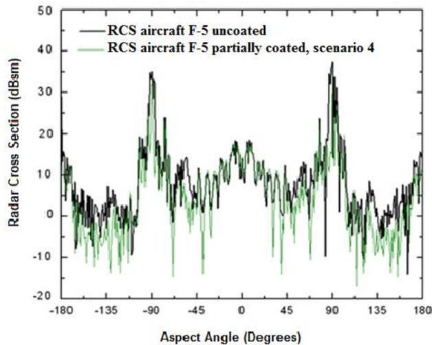
Fig. 11. Comparison between the RCS of the F-5 modified at 11 GHz, partially coated and uncoated with RAM. (scenario 4).
