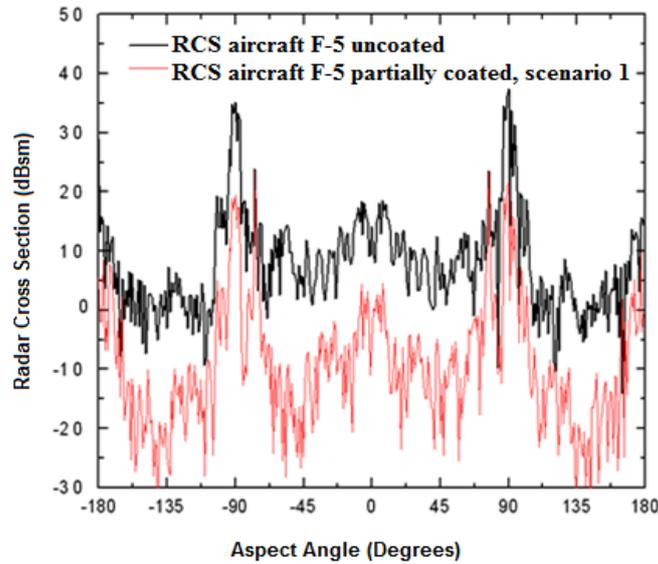
Fig. 8. Comparison between the RCS of the F-5 modified at 11 GHz, partially coated and uncoated with RAM. (scenario 1).
